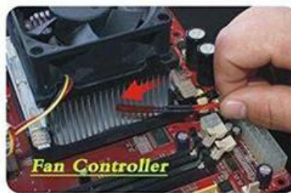
Connect the connector labeled "CPU FAN" to the connector on the CPU Fan
