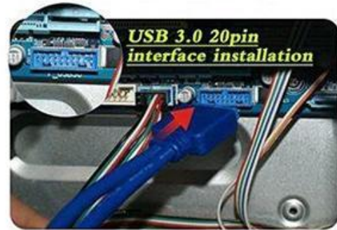
Connecting the USB3.0 20PIN to interface in motherboard
