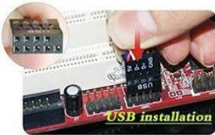
Connect the card reader USB cable to the USB port on the motherboard
