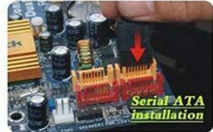
Installation connect the SATA cable to the mainboard
