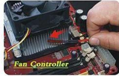
Connect the connector labeled "CPU FAN" to the connector on the CPU Fan
